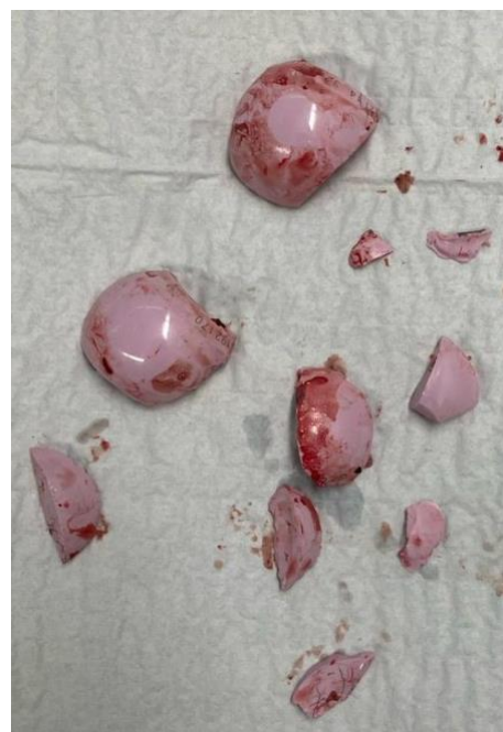
Figure 4: Clinical photo showing the broken fragments of the failed ceramic head.
